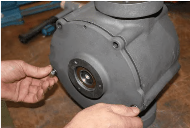
Fit bearing cover (08) with bolt (63) and washers (64).
