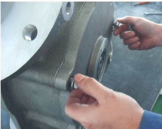
Fit bearing cover (08) with bolt (63) and washers (64).
