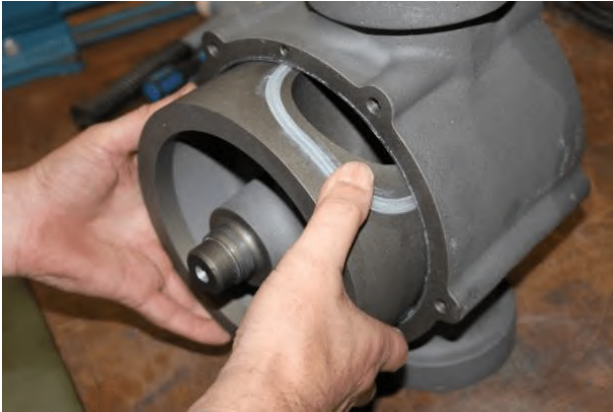
Fit end cover (03) with bolts (56) and washers (57).
