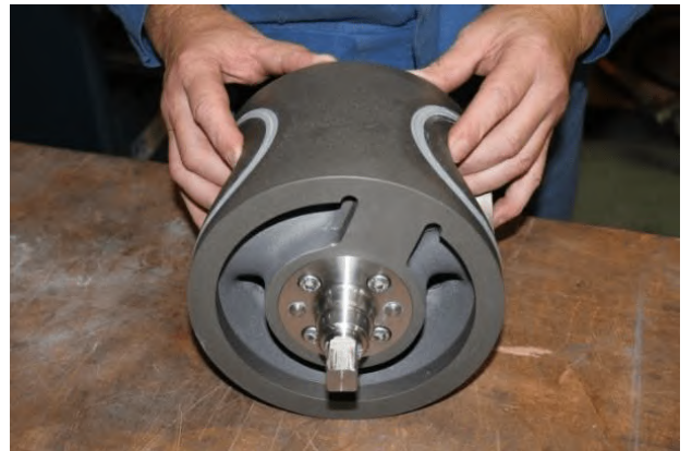
Check seal (05) for damage and replace, if necessary.
