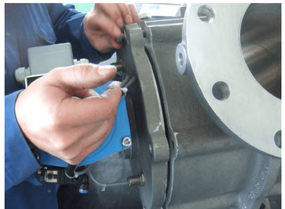
Fit end cover drive side (02) with bolt (56) and washers (57).
