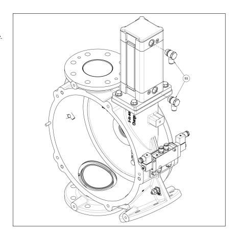
**Step 3**Disconnect the pneumatic assembly by removing its two hex bolts.
