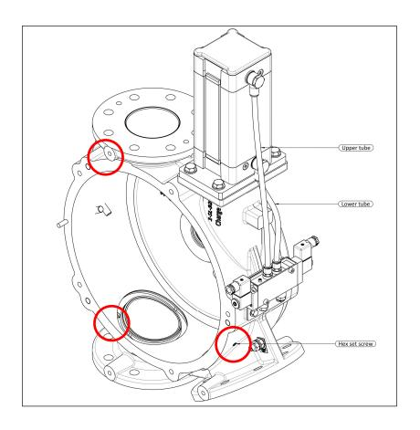
**Step 1**Remove the tubes between the actuator and solenoid valve by pushing on the coupling ends. These tubes will not be used anymore.
