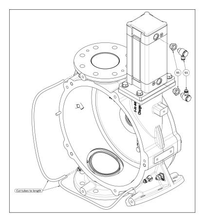
**Step 7**Install the PTD upgrade kit onto the PTD using the three new sets of bolts and washers (17&72) provided.
