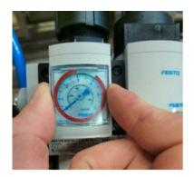
Set the front red disc (furthest from the sight glass) in the sight glass to set the upper limit to 4 bar. The range between 3 and 4 bar is now green and red outside these limits.
