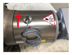
Figure 5.57: Zero speed indicator (on coupling)
