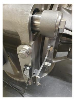
Figure 6.2: Magnetic safety switch
