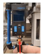
Push the arrow down/"B" button, now "OutB" (Output B), blinks at the top of the "SPEC" screen.
