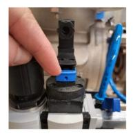
Open the pressure regulator by pulling out the round knob.
