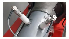
Figure 5.63: Rotor pick-ups for rotor interference detection
