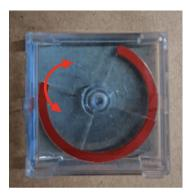
Adjust the rear red disc (closest to the sight glass) in the sight glass to set the lower limit to 0 bar.
