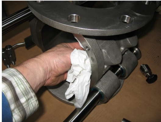
Remove two bolts used as extractors from cover.
