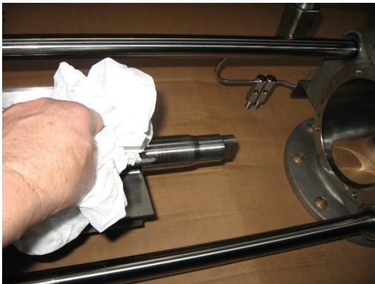
Clean rotor and shaft end.
