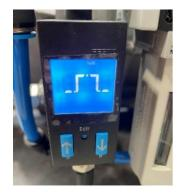
Push the "Edit" button of the flow indicator [651], "OutA" (Output A) blinks at the top of the "SPEC" (Special Menu) screen.
