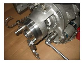
If necessary two bolts can be fitted into jacking holes of cover to enable dismounting.
