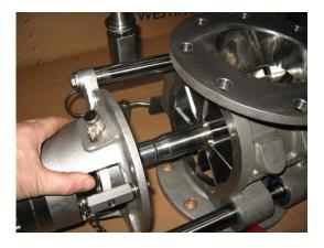
• Clean rotor surface of cover as well as head ends of rotor.
