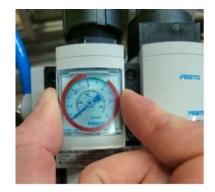
Set the front red disc (furthest from the sight glass) in the sight glass to set the upper limit to 1.5 bar. The range between 0 and 1.5 bar is now green and red outside these limits.
