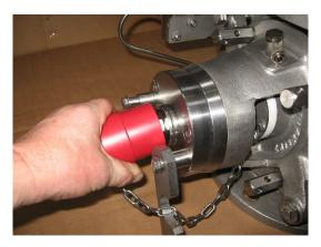
Loosen nut from locking unit (180) and remove.
