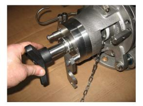
When the rotor is not correctly pulled against the cover, removal of the cover with the rotor from the body may cause damage to the body or the rotor.
