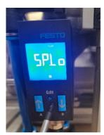
When the screen shows "SP.Hi" (Switching Point - High), set the upper limit with the arrow buttons to the flow values from the table below:
