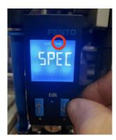
Push the arrow down/"B" button to set the upper and lower flow limit. The screen shows "\_\_\_" (Window comparator).
