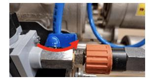
Set the pressure regulator 0.5 bar higher than the pressure inside the valve.
