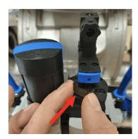
Lock the rotating knob of the pressure regulator to secure the pressure.Use a padlock for extra security.
