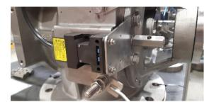
Figure 6.1: Mechanical safety switch
