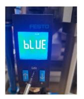
Push the "Edit" button to finish setting the flowmeter. The screen should be red and the sensor indicates a flow of 0.0 l/min.  Push the arrow down/"B" button, the screen turns red and shows "r.OFF" (Display turns red with switching status off and/or logic 0).
