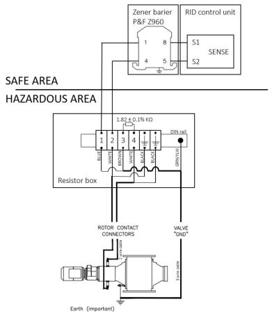
Figure 4: RID connected using a Barrier.
