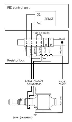
Figure 3: Sense lines directly connected to the machine.
