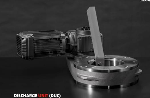
The DMN-WESTINGHOUSE discharge unit is designed to prevent product bridging at the hopper outlet (up to 176 ft<sup>3</sup>). A rotating paddle inside the hopper cone keeps the product in motion. This design is particularly beneficial when dealing with mixed products, as the rotating blade helps to avoid product separation at the hopper outlet. The discharge unit guarantees a
