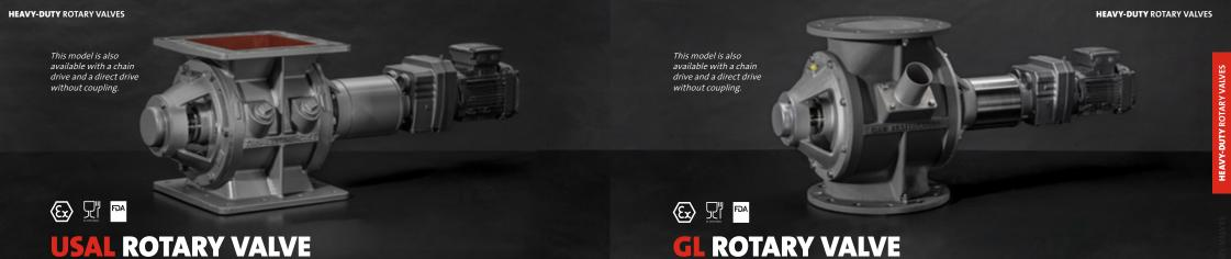
The USAL rotary valves have been designed for many applications in the metering and pneumatic conveying of products in powder and granular form. The USAL has square inlet/outlet flanges. It has an enlarged inlet, designed for applications where inlet size is more important than capacity, or for handling products that flow poorly.
