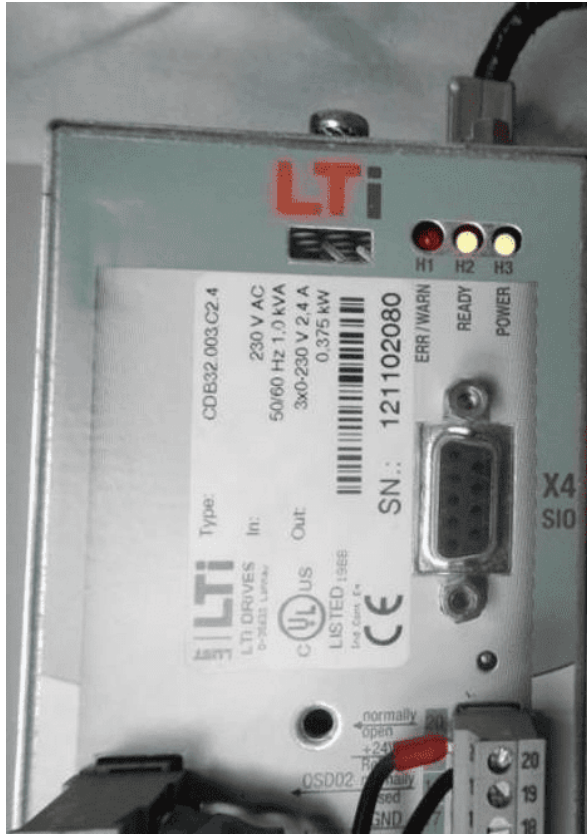
Figure 16.11: Position controller (M-TDV)
